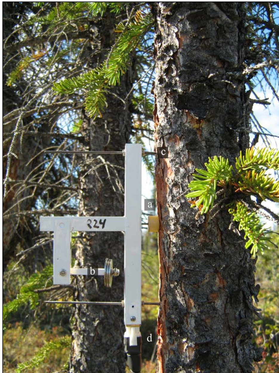
Figure 3.10. Picture of automatic point dendrometer (#13) installed on tree 32 at Blueberry: (a) sensing rod, (b) constant force cantilever, (c) steel mounting rod, (d) LVDT cable connector.
