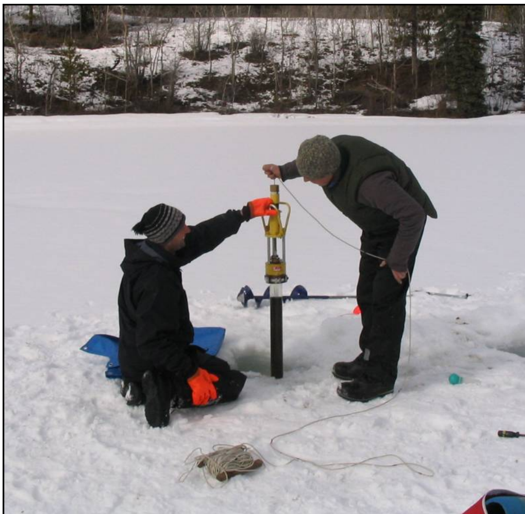
Figure 4.1: Photographs showing the collection of the surficial sediment core using a Maxi-Glew corer.
