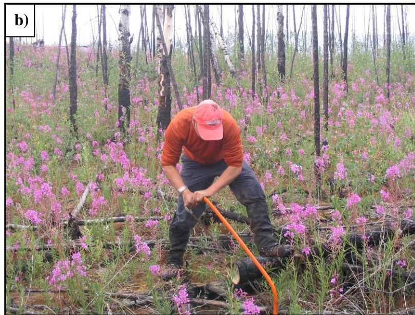
Figure 4.3: Photographs illustrating a) the collection of a tree core sample using a 14-inch Hagloff increment borer; and b) the collection of a cross-section from a charred spruce tree using a bow saw.
